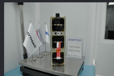
SXC3-219 ISOI ISOI RAS and Medex LLC Mass – 4 kg Purpose – Ed-Scientific sat Launch date – August 9, 2012
